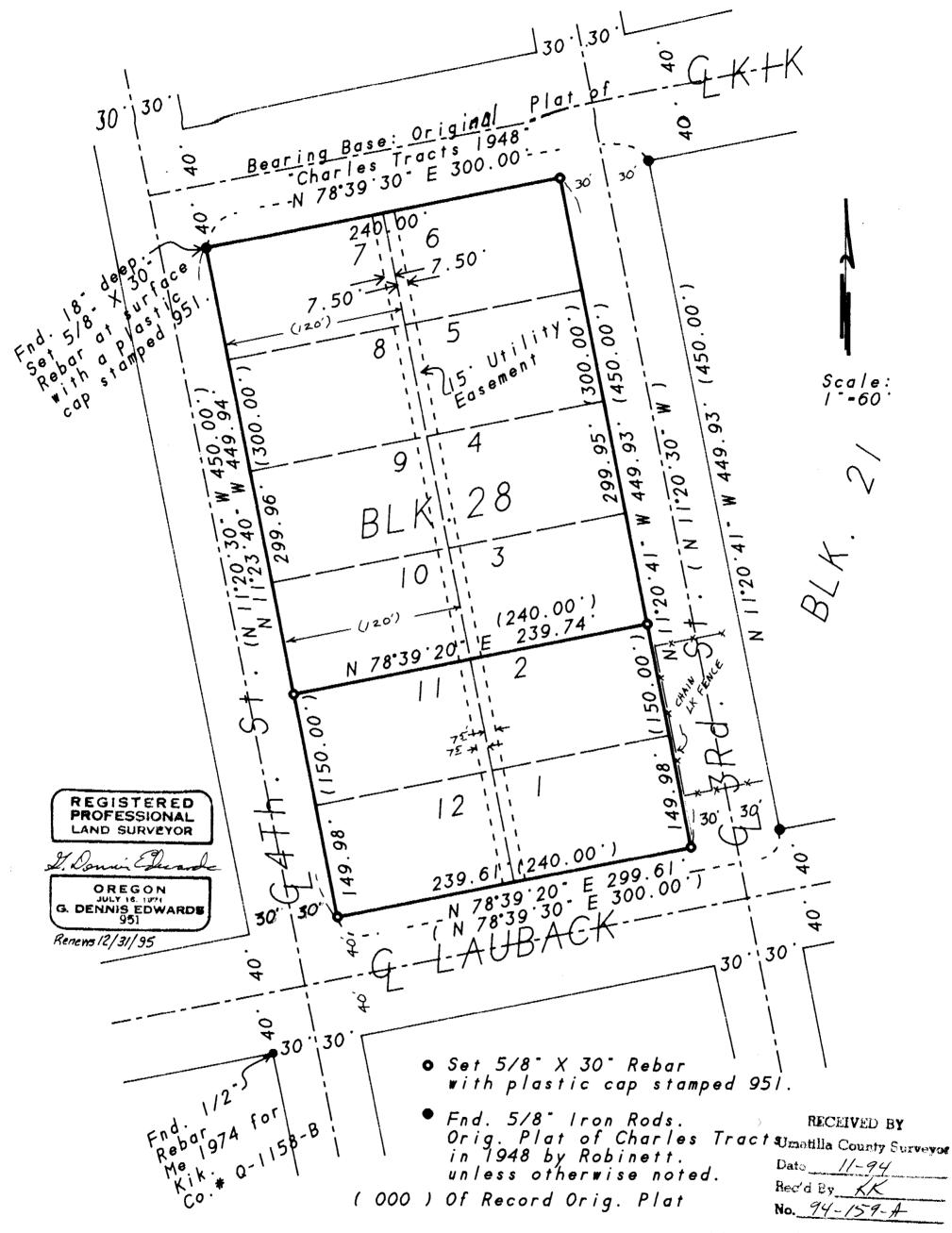
NARRATIVE: The purpose of this survey is to stake Two parcels in Block 28. "Charles Tracts" for the construction of Two Commercial Businesses. The Bearings and the Survey are based on the Original Plat of 1948 by Robinett.
