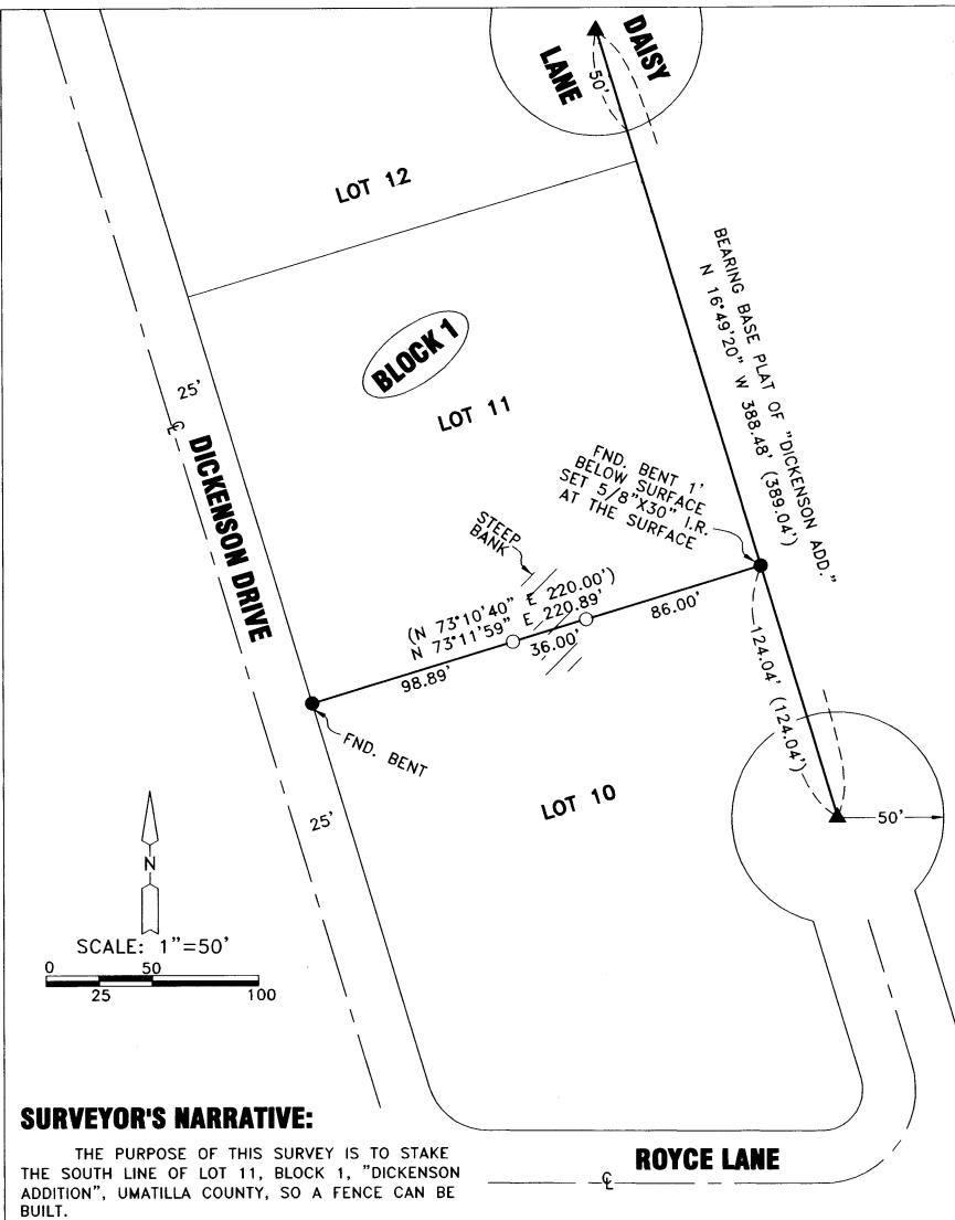
I FOUND BOTH SOUTH CORNERS AND SET IRON REBAR AT THE TOP AND BOTTOM OF A STEEP BANK.
