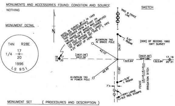
ON A STRAIGHT LINE BETWEEN THE NW CORNER & NE CORNER OF SEC. 20, AND TAKING INTO CONSIDERATION FENCE CORNERS AT THE E 1/16 AND HERE. I SET A 1"X30" IRON PIPE WITH 2 3/8" BRASS CAP STAMPED AS ABOVE. (SEE MY 1997 SURVEY FOR NAPOLITANO)
